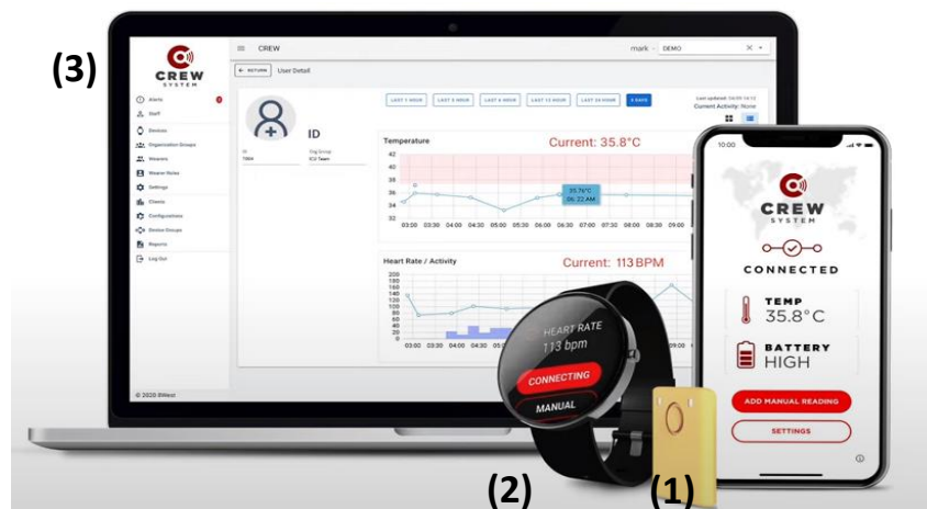
Figure 8. Overview of the main components included in the CREW system: wearable digital thermometer sensor (1), sensor platform (2), and cloud platform (3) (8 West, 2020).
