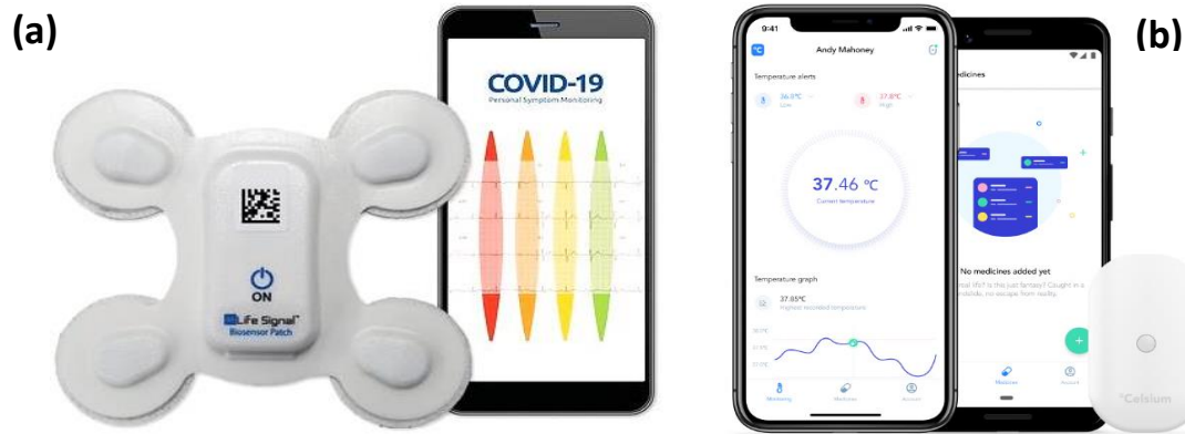
Figure 6. Smart patch developed by LifeSignals Co. for monitoring the patients' main vital signs (a); wearable thermometer armpit-placed, produced by Celsius company, placed at the armpit, to monitor the user temperature remotely (b) (Celsius, 2020).
