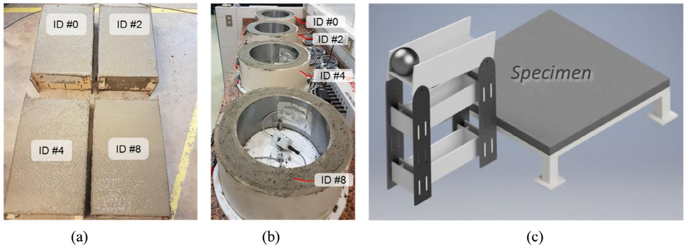
**Fig. 2.** Plastic shrinkage cracking test: (a) mortar specimens after casting; (b) age at cracking under restrained shrinkage setup for each mortar mix; and (c) impact test setup.
