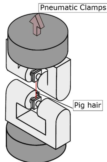
Fig. 1. Setup of pig hair tensile strength test.
