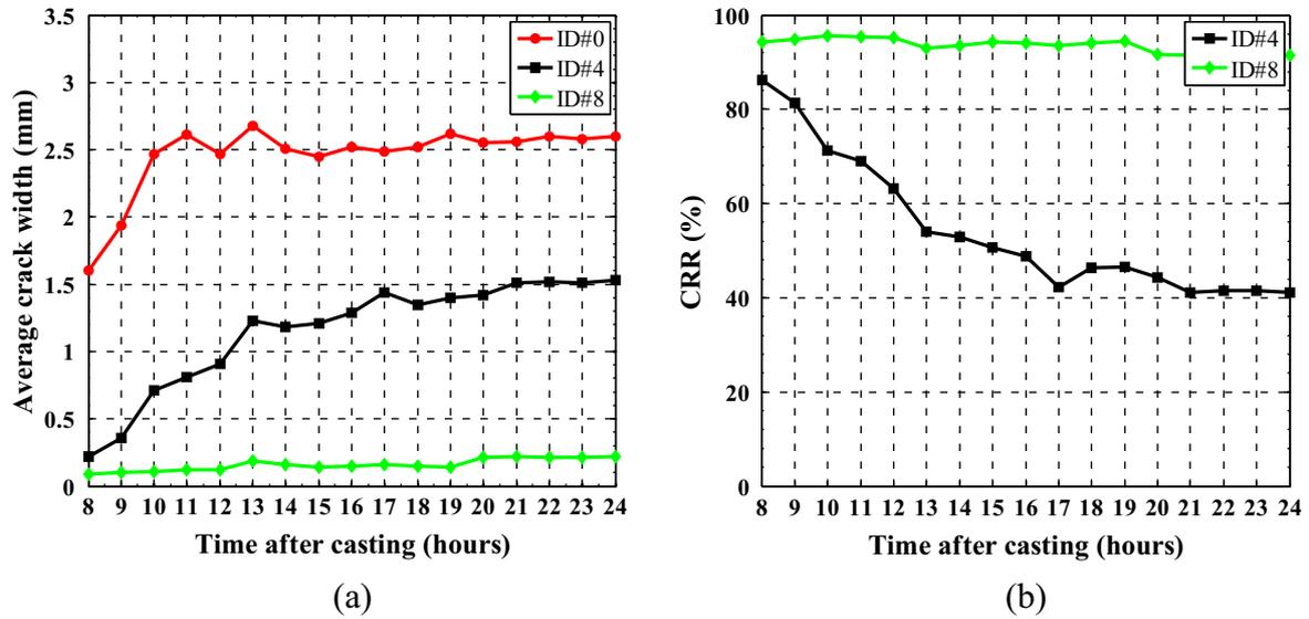
Fig. 8. Plastic shrinkage cracking tests for each mortar mix: (a) average crack width as a function of time after casting; and (b) crack reduction ratio as a function of time after casting.
