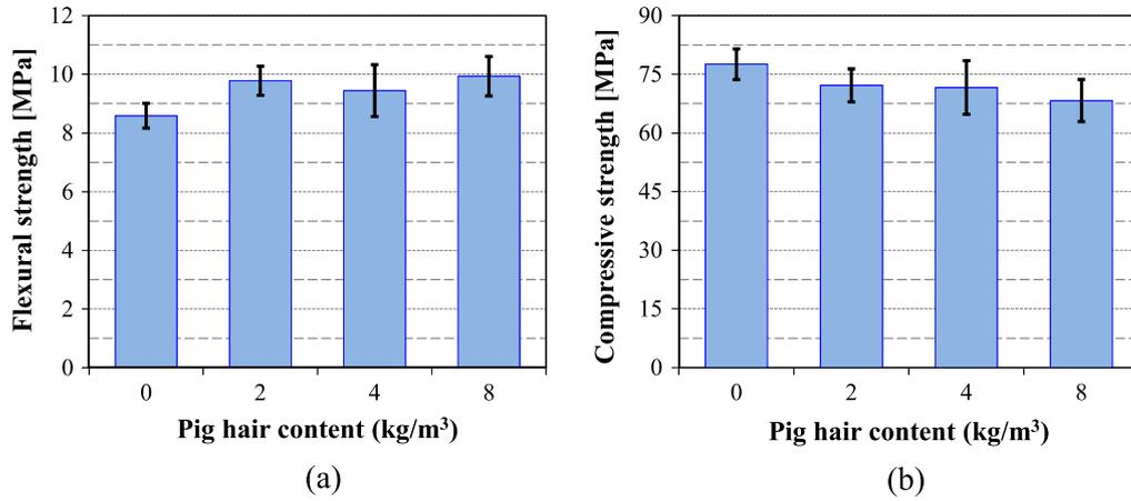
Fig. 5. (a) Flexural strength at 28 days versus pig hair dosage in kg/m³; and (b) compressive strength at 28 days versus pig hair dosage in kg/m³.
