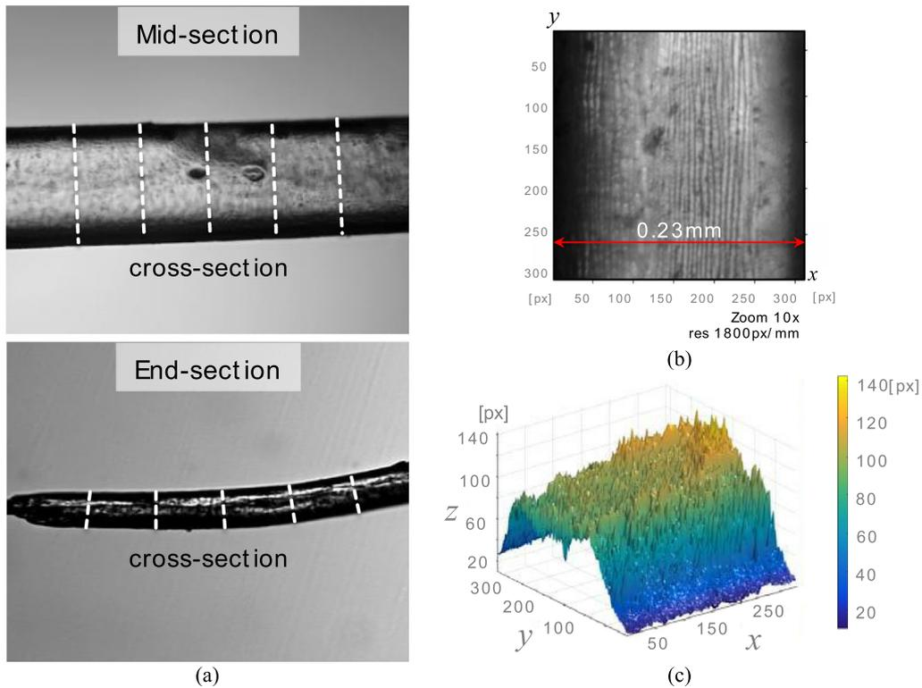
Fig. 3. Morphological analysis of pig hair for this work: (a) methodology to measure diameters at mid-section and end-sections; (b) 0.23 mm diameter pig hair: microscopy at mid-section; and (c) 3D elevation of its surface at mid-section.
