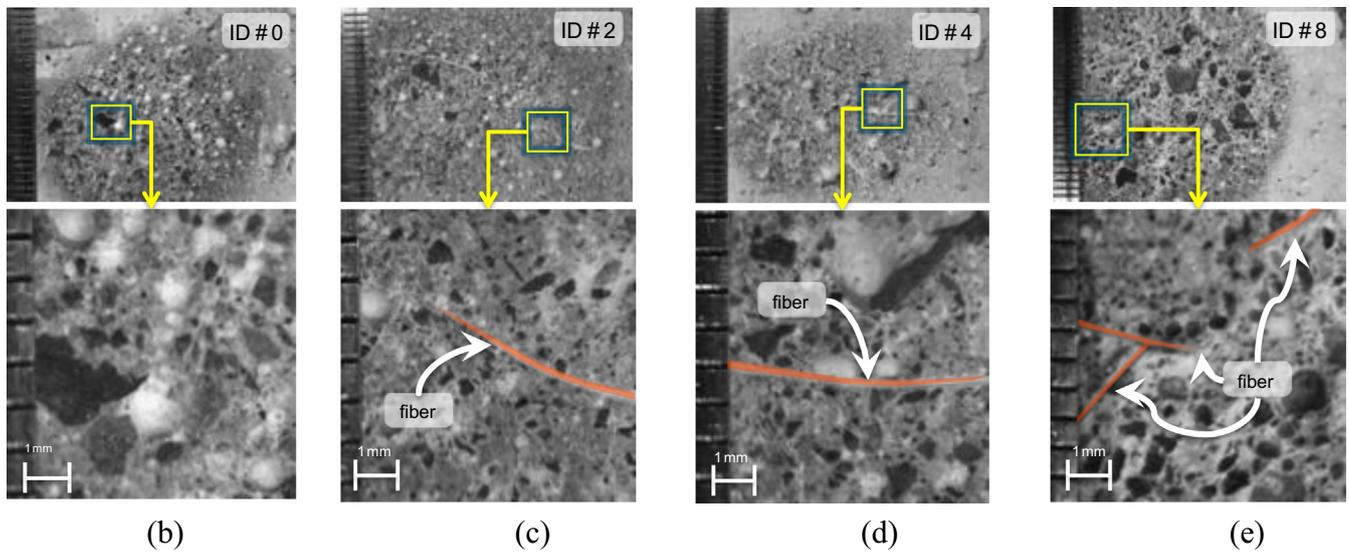
Fig. 6. (a) Percentage of mass loss at different volumes of sand versus dosage of fibers; and (b) to (e): abrasion surface of mortar with 0, 2, 4 and 8 kg/m³ of fiber respectively at 126 liters of sand (fiber digital colored).
