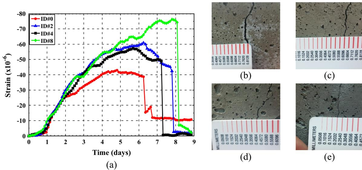
Fig. 9. (a) Strain measurements of the steel ring for each mortar mix. Measurements of crack width after ring test for mortar mix: (b) ID#0; (c) ID#2; (d) ID#4; and (e) ID#8.
