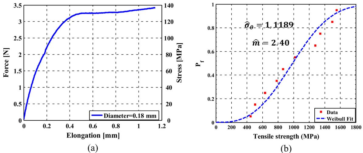
Fig. 4. (a) Tensile strength test of a pig hair; and (b) experimental data from the 10 pig hair sample tensile strength tests and Weibull cumulative distribution function obtained using the method of maximum likelihood.
