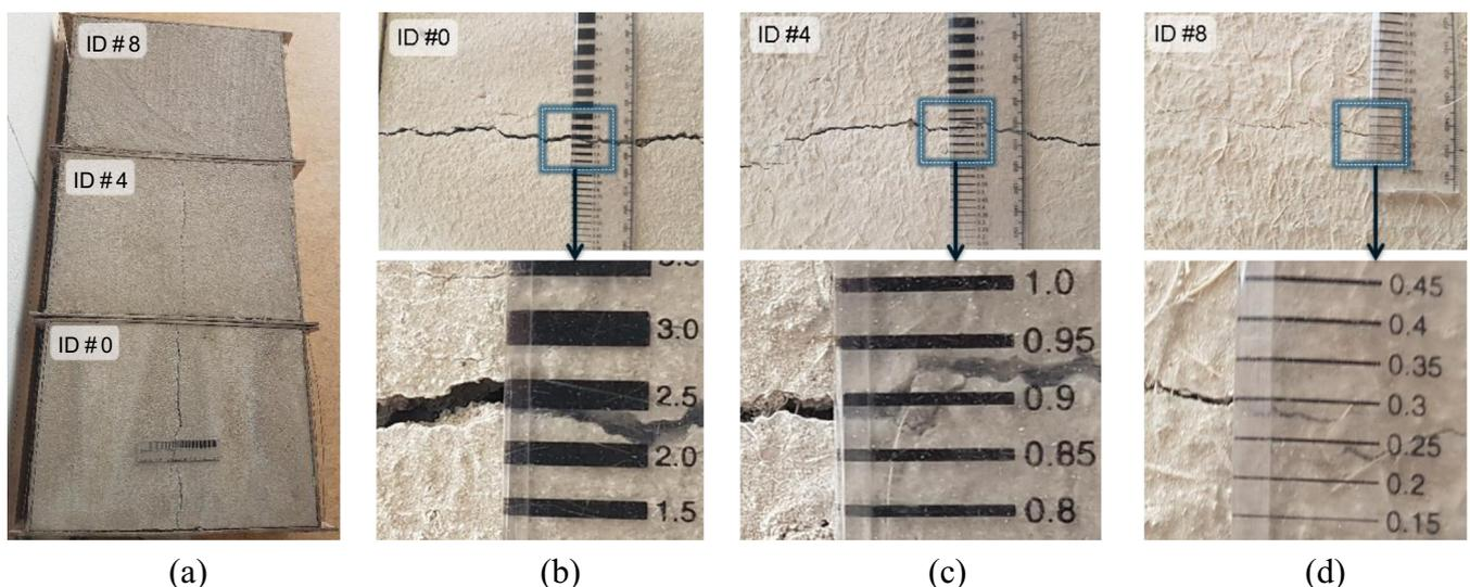
Fig. 7. Plastic shrinkage cracking test: (a) samples after-testing from bottom to top mortar specimens ID#0, ID#4, and ID#8 are showed; (b) mortar specimen ID#0 with crack width of 2.5 mm; (c) mortar specimen ID#4 with crack width of 0.9 mm; and (d) mortar specimen ID#8 with crack width of 0.3 mm.
