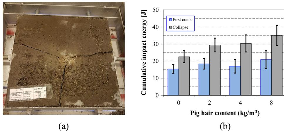
Fig. 10. Impact strength: (a) mortar mix ID#8 slab specimen tested; and (b) mortar mixes cumulative impact energy at occurrence of first crack and at collapse.
